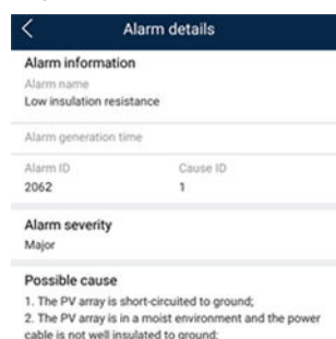
Figure K-1 Alarm details
