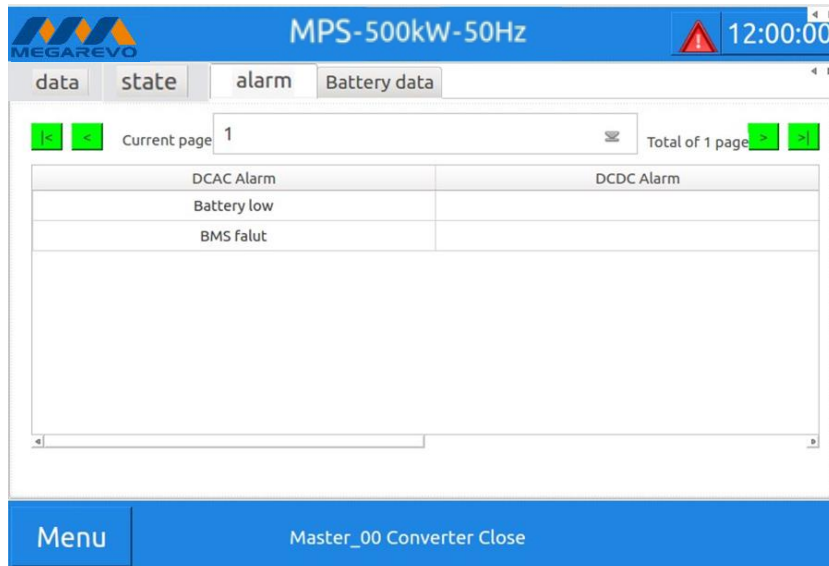
Figure 8-3 Alarm item list
